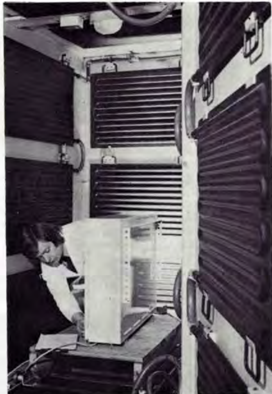
Testing a storage radiator's performance in a 'calorimeter' chamber.
