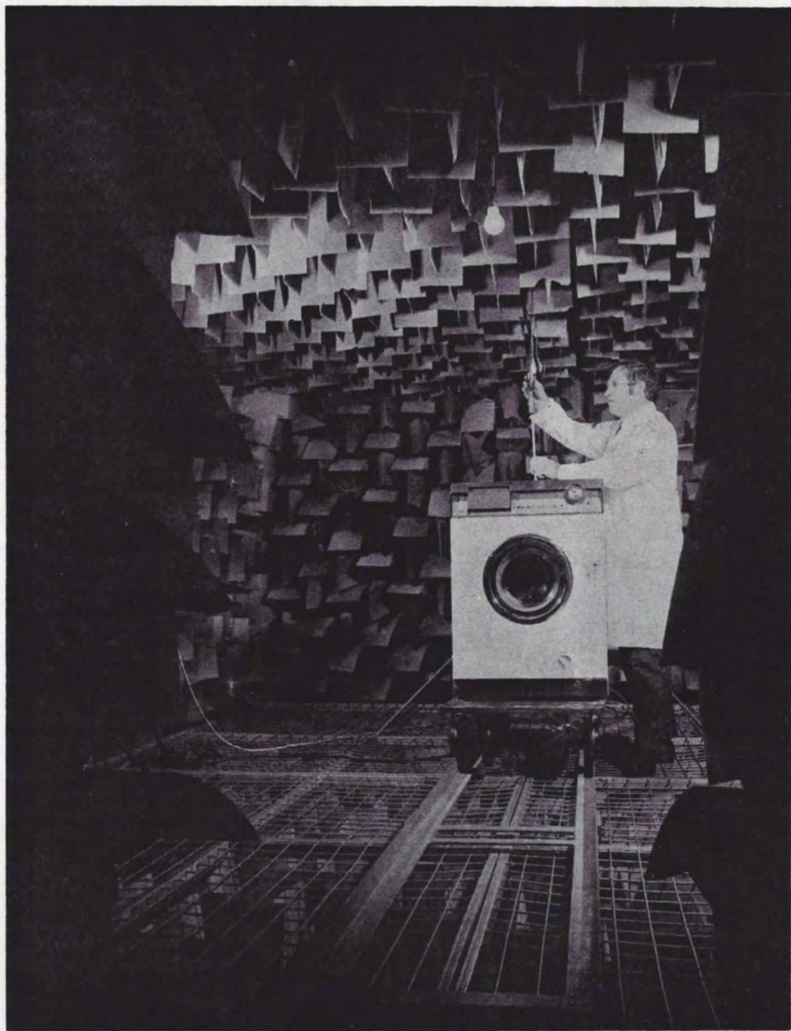
The noise measurement chamber could have come straight from "Doctor Who." Wedge shaped pieces of foam, covering walls, floor and ceiling, kill all echoes stone dead, making accurate measurement of noise from appliances possible.
