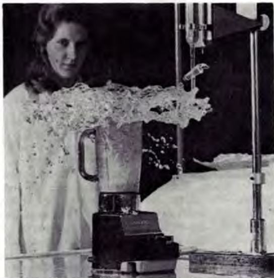
Safety test on a blender, with the jug lid removed. Appliances must be able to stand up to various misuse tests of this kind.
